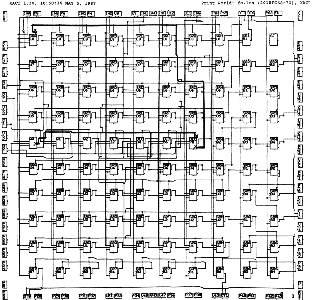
Figure 6. Layout Diagram of “Corner Bender” Circuit on LCA Device of Size 10x10
